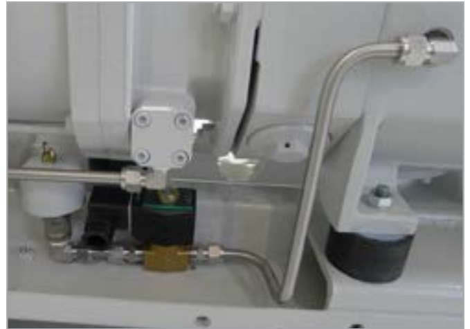
Fig. 3.13 LEYVAC with gas ballast kit installed (24 V)
